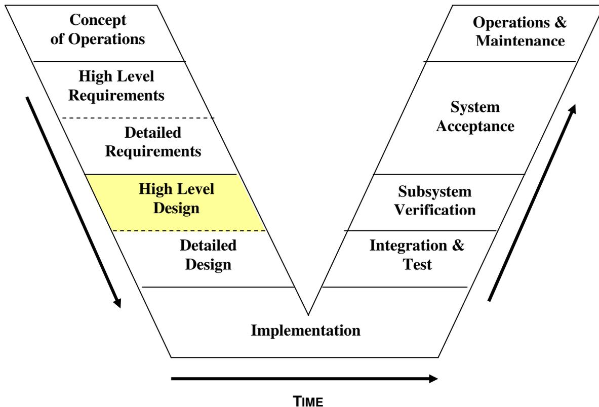
Figure 1 – “V” Diagram of Systems Engineering<sup>1</sup>
